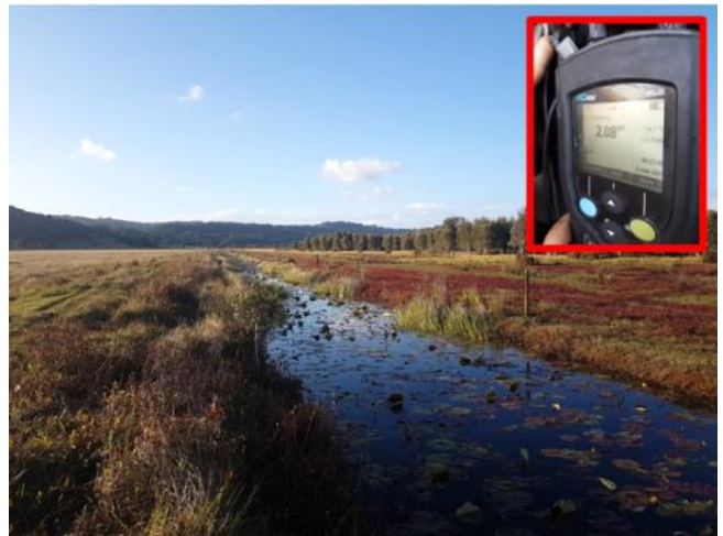
16: Jumbo Drain, where pH comparable to lemon juice (pH=2) was observed
